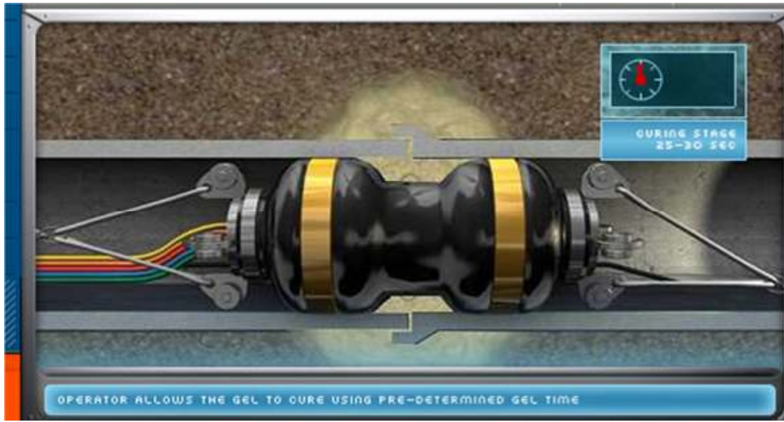
Figure 4.2 – Chemical grouting of Sewer Pipeline (source: Avanti International)
