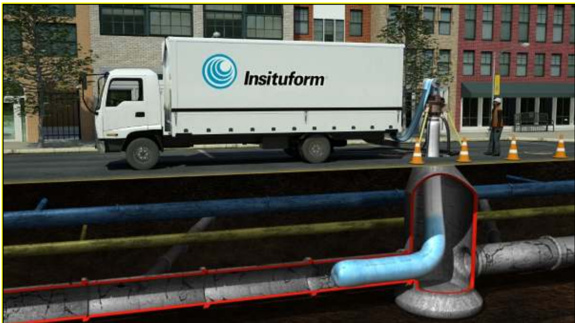
Figure 4.1 - Installation of CIPP Liner (source: Insituform Technologies)
